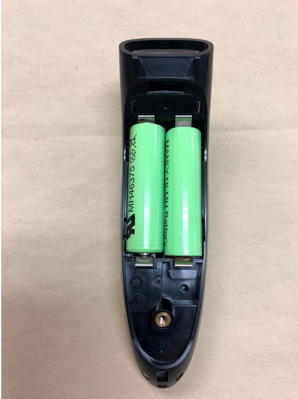
Figure 5 – S7xx Series – Rear Internal Showing Batteries
